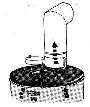
Open the smoke damper and draw the ash box open for 5-10 cm. See that sufficiently combustion air comes into the sauna either from the valve or through the door. Note that the sauna is not ready for bathing until the heating has been stopped and the löyly shutter is opened.
