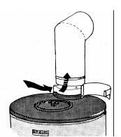
If there is no ventilation valve in the upper part of the sauna, the sauna can when necessary be ventilated by closing the löyly shutter and by opening the flap in front of the smoke damper. This can also be used for drying the sauna after bathing. The smoke damper must then be shut (picture).
